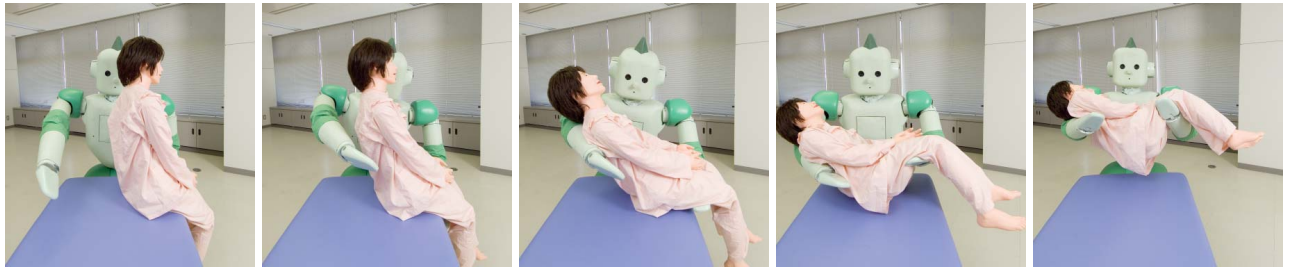
Fig. 9 Experimental results of holding up a dummy by RI-MAN
