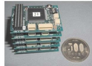
Fig. 9 Local controller “C-CHIP”
